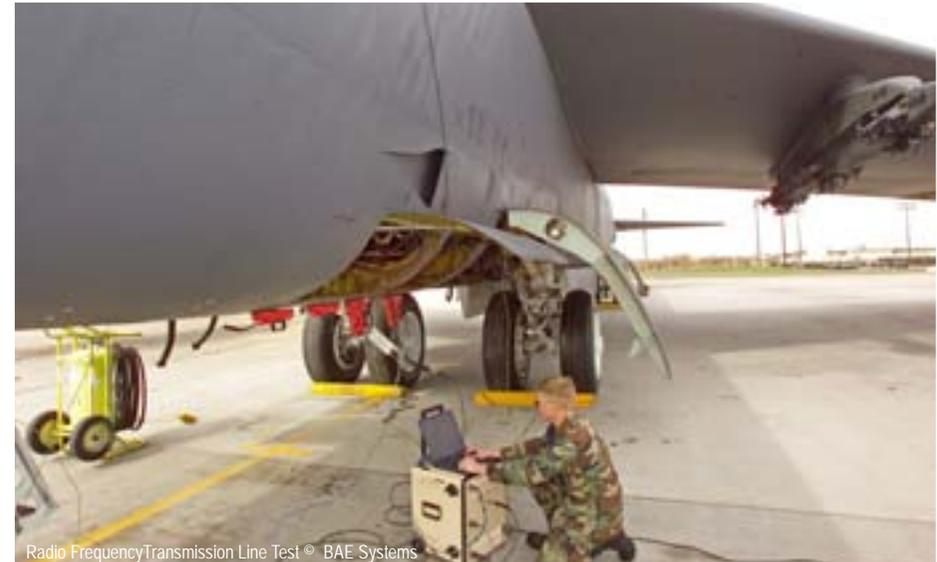
Radio Frequency Transmission Line Test © BAE Systems
