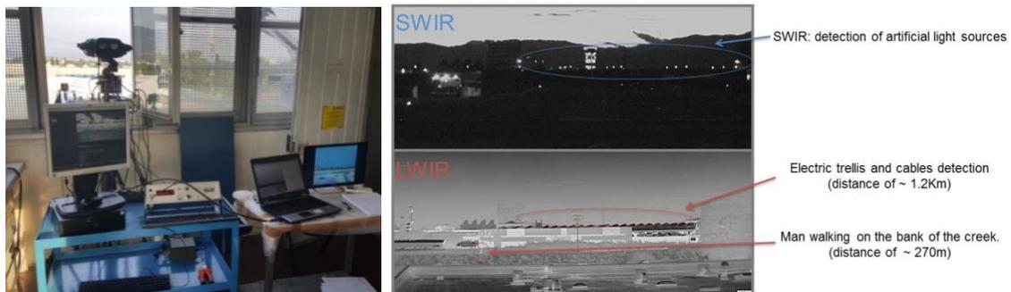
Figure 3 – Set-up for simultaneous image acquisition in different spectral bands at Leonardo premises (left) and comparison of imaging capabilities in different spectral band (right), in urban scenario, during nighttime. Images acquired during the experimental tests.
