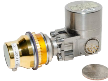
Figure 6. RED HOT FPA integrated in SWaP IDDCA with RMs1 cooler from Thales Cryogenics.
