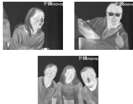
Figure 7. Imaging with RED HOT FPA (640x512 pixels, 15 \mu\text{m} pitch), operated at 110 K. Temporal NETD = 21mK, spatial NETD = 7 mK, F/4, and 10 ms integration time.
