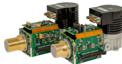
Figure 9. General view of IRnova's IDDCA for SF6 gas detection in quarter VGA and VGA resolution with F/\text{numbers} of 2.0 and 1.2, respectively. The IDDCA share most of the envelope parts and the 0.5 W cooler. The operating temperature is 57 K.
