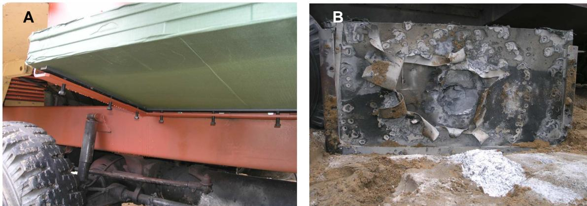
Add-on armour before (A) and after (B) EFP mine attack.
