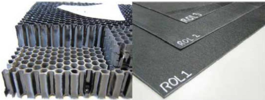
Example of honeycomb (left) and fiber reinforced laminate (right) impregnated with radar absorbing material.
