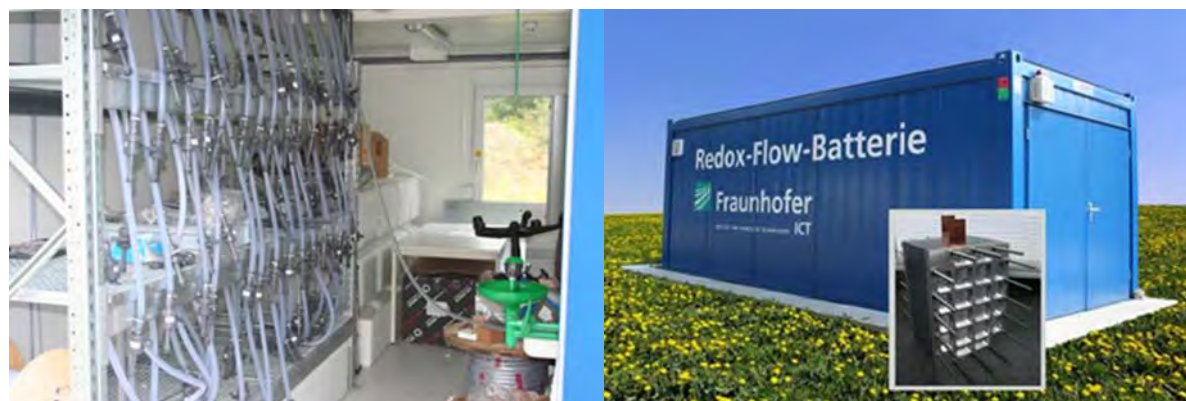
Figure 4: Development of Military Battery Systems at Fraunhofer ICT under contract of WTD 51 - Wehrtechnische Dienststelle für Pionier- und Truppengerät (17 kW VRFB, 24 Stacks (600 cm 2 , 22 cells), current max. 360 A; potential 175 V, power 34 kW, powerdensity 30 kWh)
