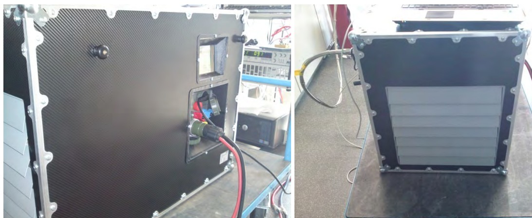
Figure 1: Front view (left) and view of the exhaust shutters (right) of the fuel cell generator.
