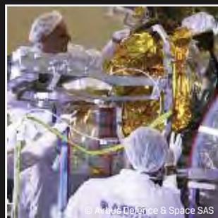
The Tesat Spacecom laser communication terminal - integrated on the Eutelsat-9B satellite at Airbus Defence and Space, Toulouse
