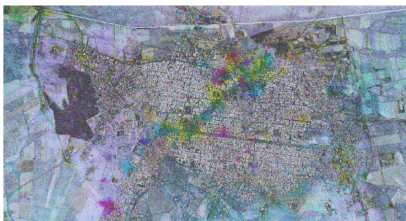
Multi-coherence product from the execution of a workflow for damage assessment COSMO-SkyMed image © ASI 2017
